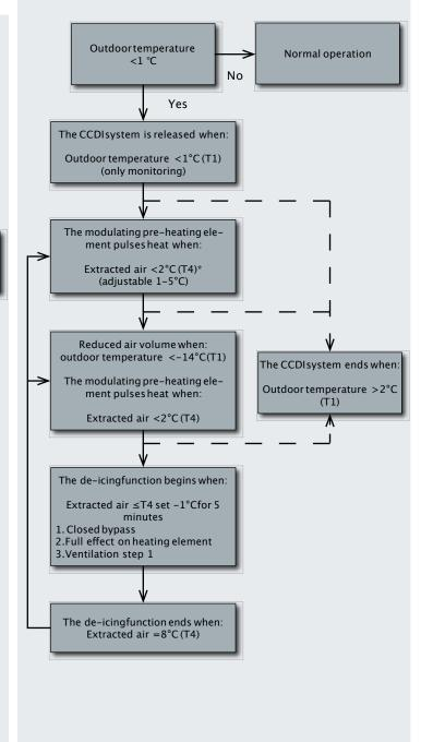
NB! All temperature settings are adjustable. On adjustment, they must be matched to the conditions in the home and the local climate.
