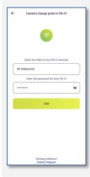
Apple iOS devices – Privacy rules prevent a list of networks being shown. However, if Location Services have been accepted (when first using the App) and the smartphone is connected to your Wi-Fi network, the App will automatically suggest the Wi-Fi network you were last connected to and just require the password.
