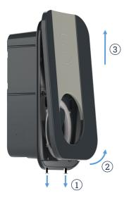
Loosen the two screws fitted along the bottom edge of the fascia with a no 1 Posi-drive screwdriver ① (no need to remove the screws ) and lift the cover away from the base at the bottom ②. Remove cover by pulling upwards and unhooking at the top edge ③.
