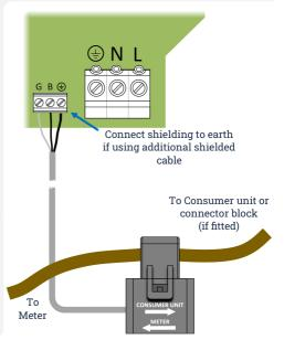
3. <u>Install clamp.</u> Open the measurement clamp and position around the previously identified supply cable, observing the correct orientation marked on the clamp. Close the clamp around the cable and ensure that the latch is engaged.
