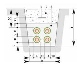
SLW 30 300 kN total load as per DIN 1072; if subject to higher traffic loads (e.g. SLW 60), a load-distributing superstructure as per RStO75 is required. With no traffic load, the minimum trench depth T can be reduced by 20 cm.
