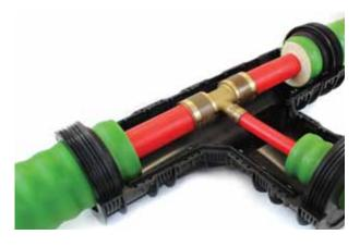
(1) Position the lower shell sleeve and ensure that the sealing rings are precisely located (see picture). PLEASE NOTE: The lower shell does not have the plug holes.
