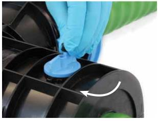
(8) After at least five minutes has elapsed, seal the openings with the rubber stoppers (see picture).
