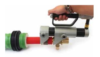
(3) Insert the PEX-LOK fitting (tee, elbow or straight coupling). Locate the clamping jaws on the tool and clamp onto the joint. For dimensions over 40mm, a lubricant of petroleum jelly must must be used in the area of the compression sleeve.
