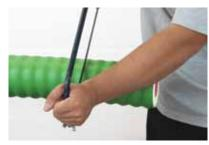
(2) Cut the casing pipe with a saw.
