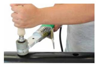
(14) Using a pre-heated electric fusion welding tool, the welded plugs need to be put into the heater, with the male end of the heater placed into the joints filler hole. When heated, the plug can be pressed into place in the hole with hand pressure until there's a visible 2mm bead melt on both the plug and hole. Repeat this process for the second hole.
