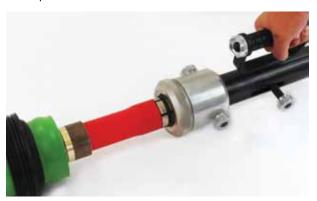
(2) Expand the pipe end twice – offset by approximately 30°. Ensure that the compression sleeve is slid well back from the area being expanded.
