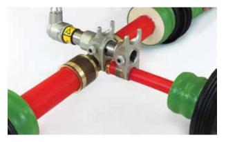
(6) If creating a Tee-branch connection, clamp the third pipe. It may be necessary to make room for the clamping tool as discussed in step (4) above.
