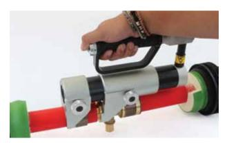
(5) Clamp the second pipe. If this is a straight or 90 degree coupling, then the connection is completed.
