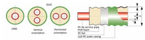
Hiline Flex in coils: Dimensions: HF 25/76 - 140/202
