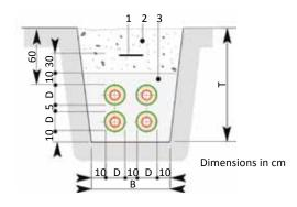
SLW 30 300 kN total load as per DIN 1072; if subject to higher traffic loads (e.g. SLW 60), a load-distributing superstructure as per RStO75 is required. With no traffic load, the minimum trench depth T can be reduced by 20 cm.
