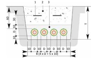
Installation depth: Max. installation depth: 2.6 m Our approval is required for installation at greater depths. 1 Pipe warning tape; see sheet HF 4.4.3
