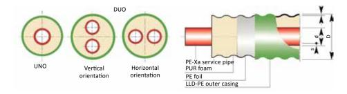
Hiline Flex in straight lengths: Dimensions: HF 160/250
