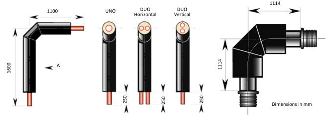
Please Note: Hiline Flex pre-insulated bends in dimensions 140/202 and 160/250 are pre-insulated steel, fitted with PEX-LOK compression connections at each end – as detailed in section 4.2.1.4.
