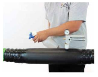
(10) Apply an air pressure test of 0.2 bar for 15 minutes and check for air tightness with soapy water on all joint areas - ensuring there is no drop in pressure. Remove the air test equipment and bore a second 25mm diameter hole approximately 100mm the other side of the centre line on the top of the oversleeve.
