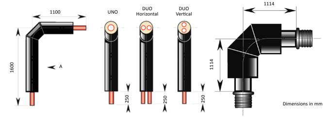
Please Note: Hiline Flex pre-insulated House Entry bends in dimensions 140/202 up to 160/250 are constructed with pre-insulated steel with pre-installed PEX-LOK compression connections as detailed in section 4.2.1.4. These fittings are also Steel grade St 37.0 P235GH TC1 - Coated with heavy-duty corrosion inhibiting compound Ardrox AV15.
