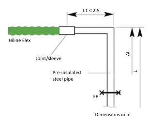
Static design of the Z-bend according to expansion variable  $\Delta l.$
