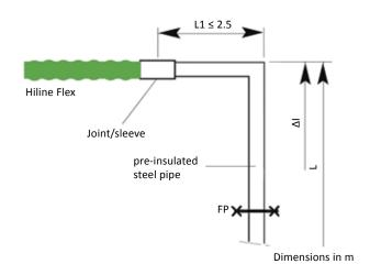
Static design of the Z-bend according to expansion variable  $\Delta {\sf I}.$
