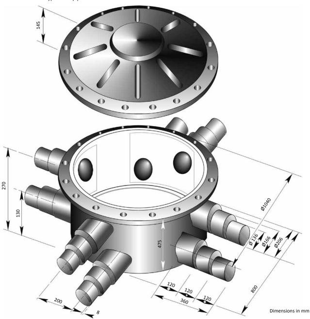
**Heat Shrink Entry Seal for Chamber Exit**
