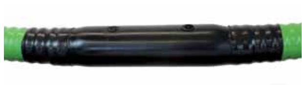
PLEASE NOTE: The heat-shrink joint and foam must be stored at a temperature below 25°C and kept out of direct sunlight. The installation of this joint must only be carried out in dry conditions and when ambient temperatures are over 5°C. Failure to comply with this may affect the integrity of the joint.
