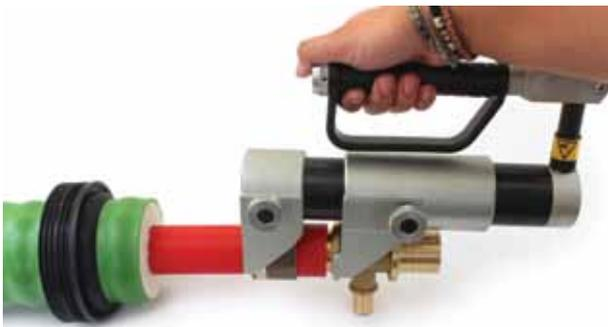
(3) Insert the PEX-LOK fitting (tee, elbow or straight coupling). Locate the clamping jaws on the tool and clamp onto the joint. For dimensions over 40mm, a lubricant of petroleum jelly must be used in the area of the compression sleeve.
