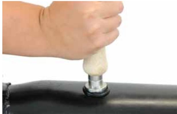
When completed and cooled, the plug should protrude no more than 1-2mm.
